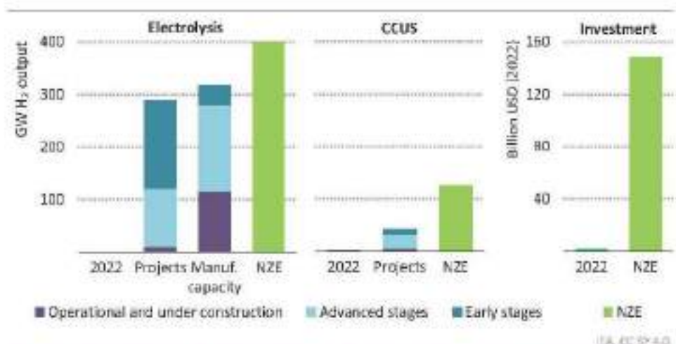
Figure 3.24 Potential low-emissions hydrogen supply capacity from electrolyser and CCUS projects and investments in the NZE Scenario, 2022 and 2030
